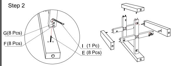
Place one end of each cross frame over the threaded rod until you can see it appear in the round hole near each end of the cross. Place the half moon and nut over the end of the threaded rod and tighten. Repeat this process for the top leg and then again for the left and right legs. Tighten all the nuts against the half moons at each connection point.
