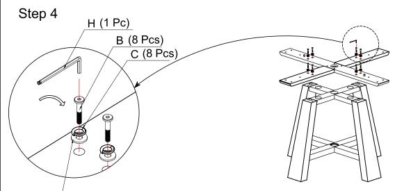
D (8 Pcs) place the flat cross frame (4) on top of the legs and insert bolts (B) together with washers (C&D) into their holes half tight at first. Fully tighten only when all the bolts have been successfully inserted into their holes.
